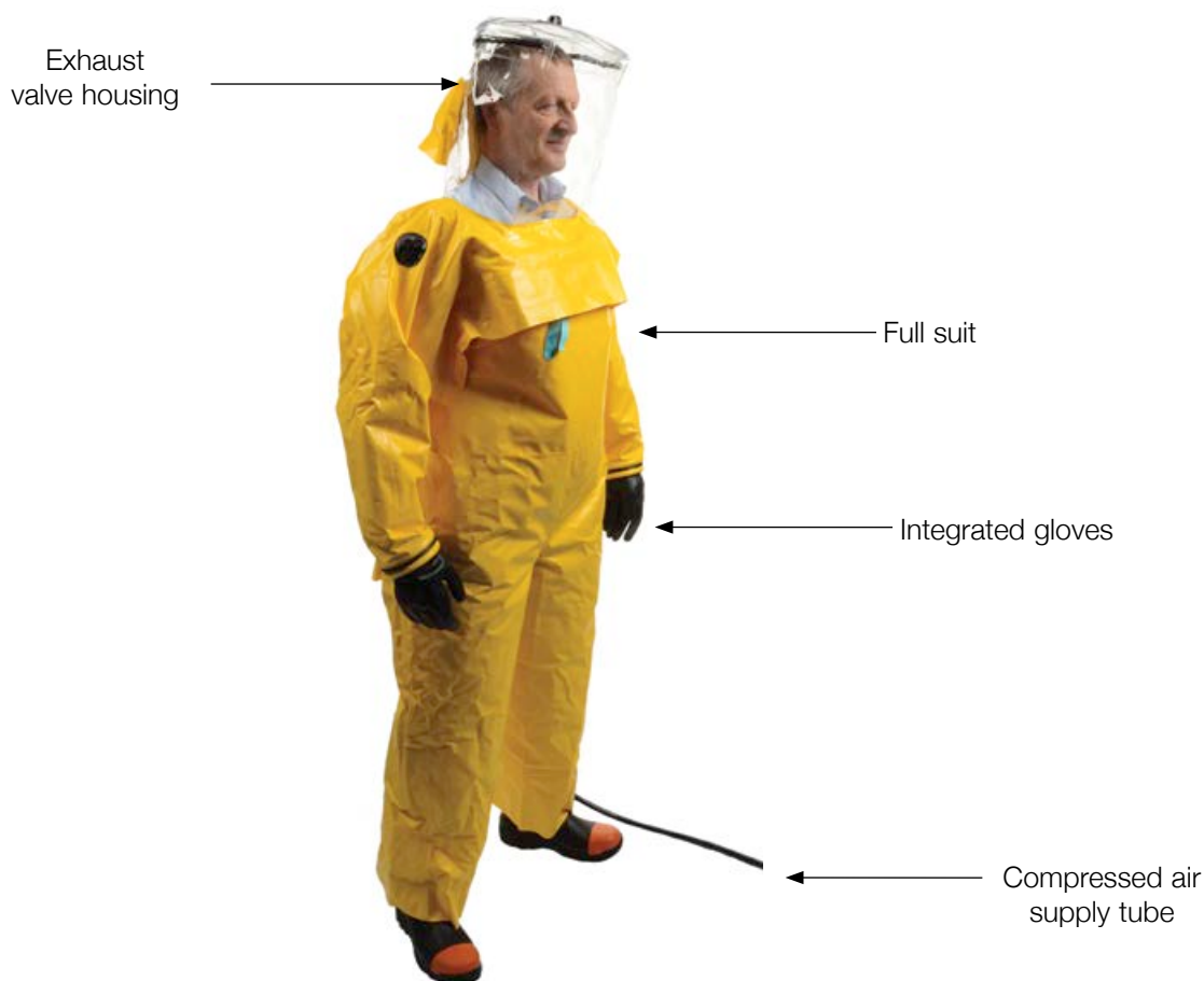
Figure 20 Constant flow airline breathing apparatus with full suit
